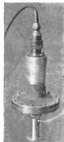
Above: "Optical potentiometer" developed at R.A.E. for use in space vehicles, including U.K.3.
